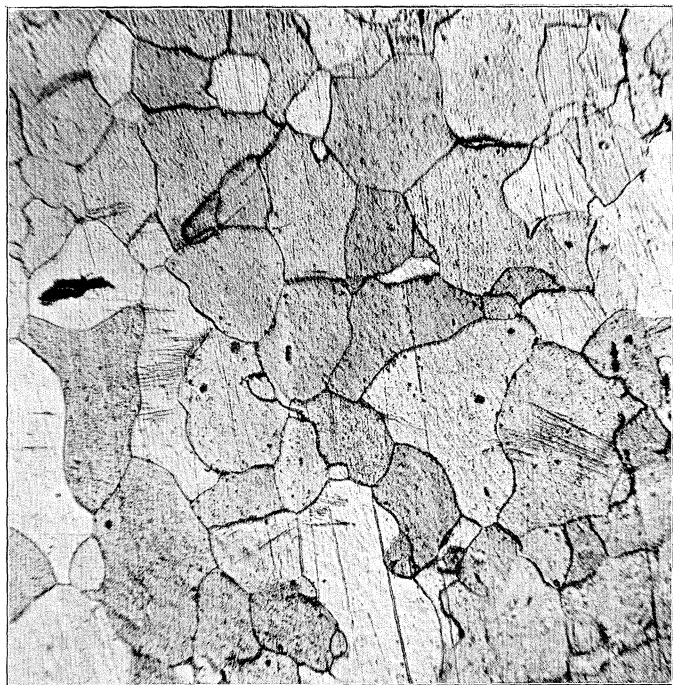
Fig. 3. Specimen of Swedish iron after 5000 reversals of a stress of 14.3 tons per sq. inch. \times 150 .
