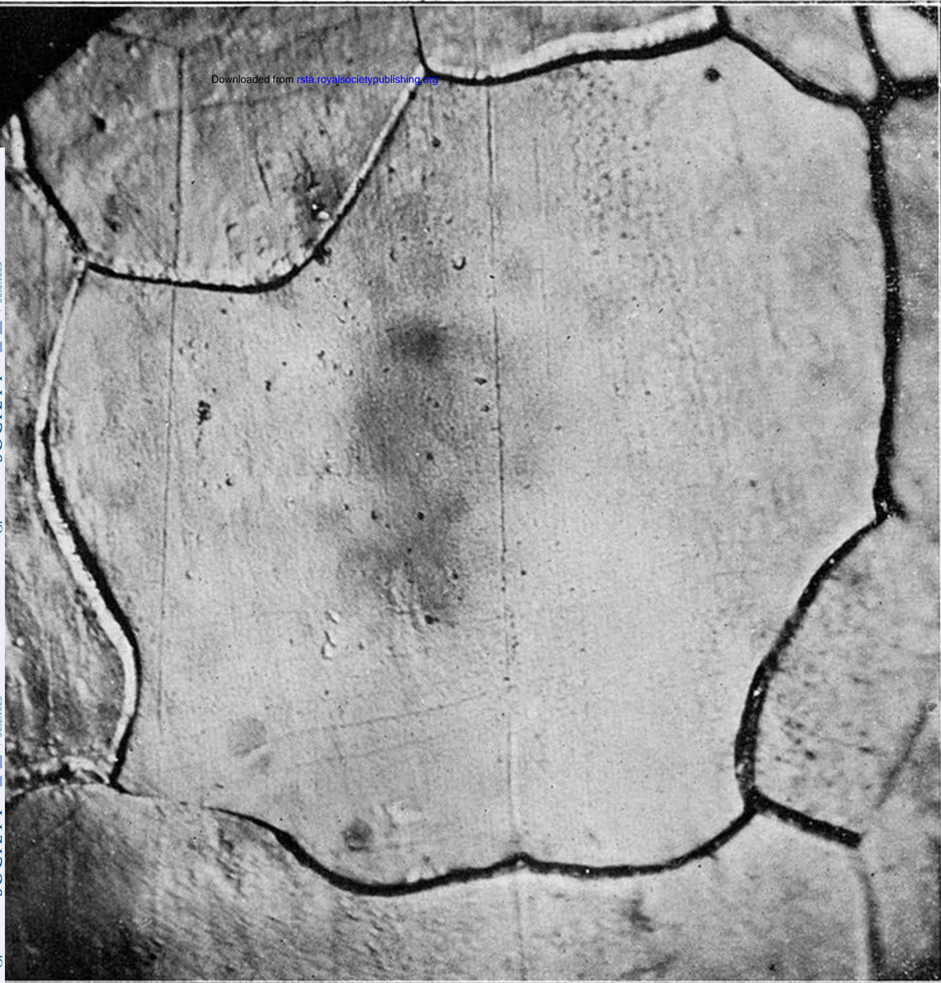
Fig. 9. Specimen after 1000 reversals of a stress of 12.4 tons per sq. inch. \times 1000 .
