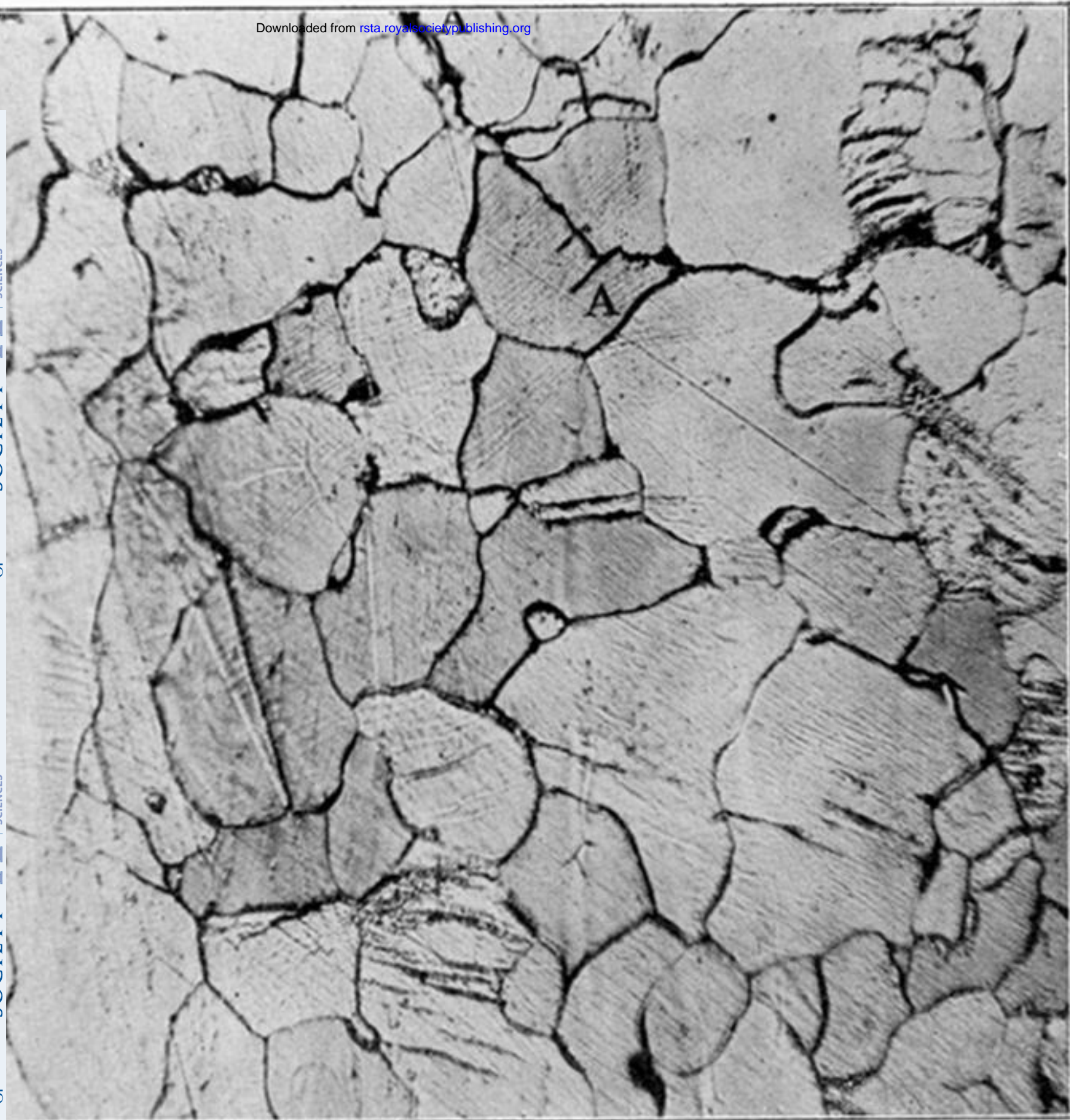
Fig. 6. Same after 70,000 reversals and re-polishing and re-etching. \times 150 .
