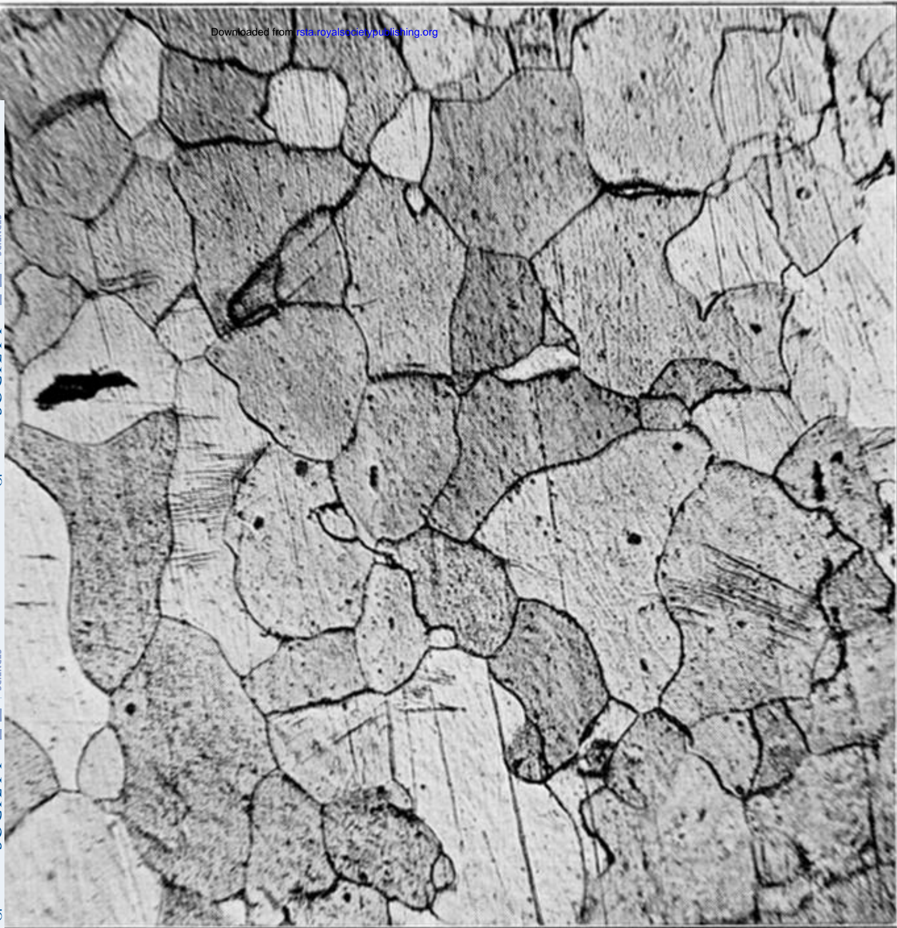
Fig. 3. Specimen of Swedish iron after 5000 reversals of a stress of 14·3 tons per sq. inch. \times 150 .
